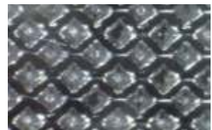
Anilox roll after Special Blade Clean wash
